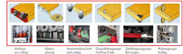
Vorfräser pro milling, Kleben gluing, Kantenendschnitt end cutting, Doppelfrägaggregat finishing R side, Zierklingenaggregat flat scraper, Polieraggregat buffing
