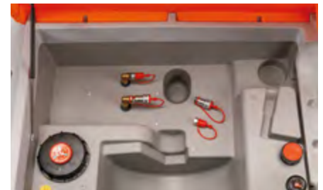
CUBE Mobil 980 generator tank with 2 connections
