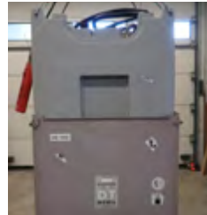
Replacement of inner tank
