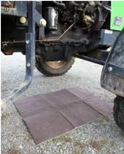
Use of the oil suction carpet from the Cemsorb emergency set Agrar
